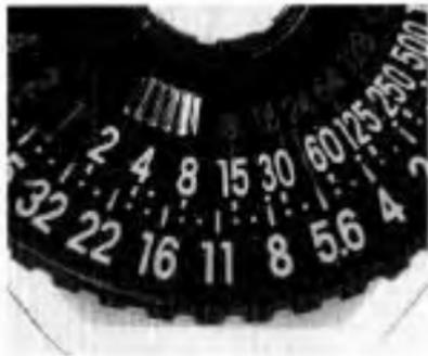
Note: Some cine cameras possess faster exposure times due to a narrower rotating shutter angle (angle of light transmitting portion). It is important to know the accurate film speed versus shutter angle value for your camera in order to determine proper exposure. Refer to the camera operating instructions, maker's catalogue, etc. for shutter speed information.
